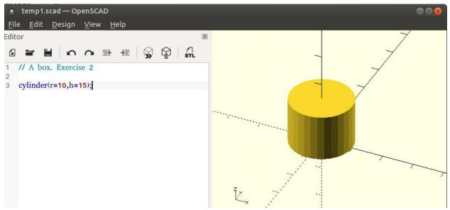
A cone is made by defining a different radius at the bottom and top of the cylinder.
