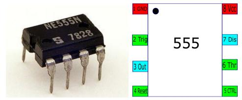
A 555 timer chip can be used to create one pulse of electricity after some interval, or can be made to oscillate and give repeated pulses.
