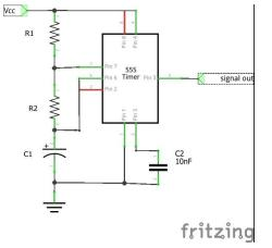
The frequency f of the pulses is  $f = \frac{1}{ln(2)C_1(R_1+R_2)}$
