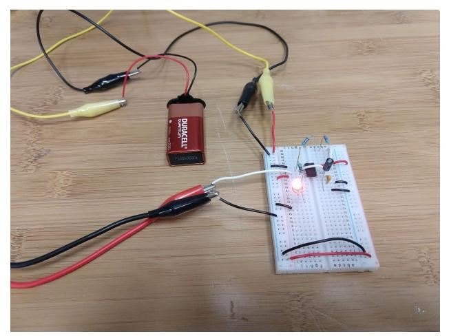
If time permits, solder the 555 timer astable timer circuit to a perf board.
